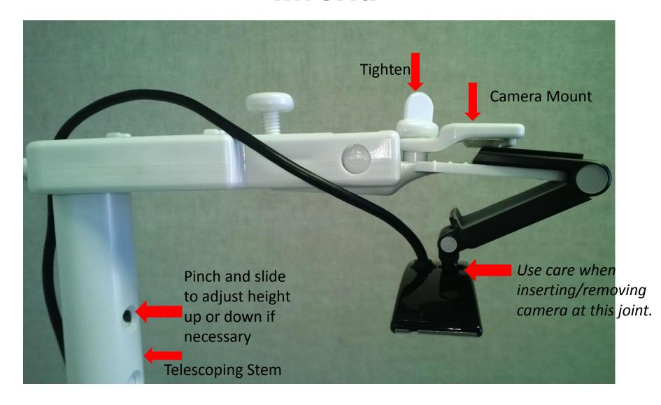
The **Telescoping Stem** is height adjustable, if necessary. Assembled at its lowest height setting both kworld & Logitech camera kits should display the bubble sheet as shown below.
